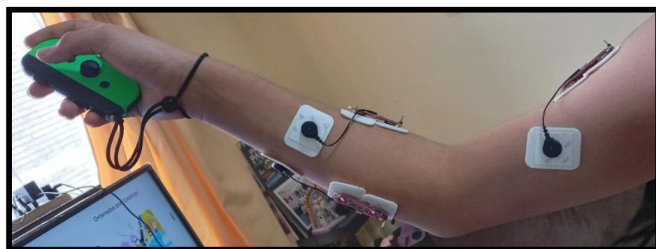
Figure 6. Setup to analyze multiple muscles
