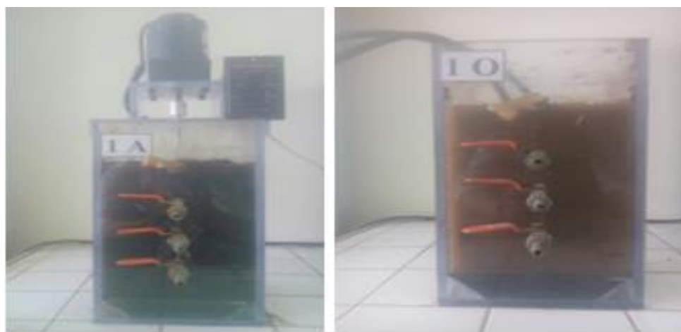
Fig 2.9: Anaerobic tanks and SBR used in the study
