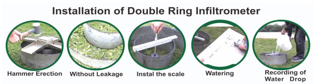
Figure 2: Instalation of Double Ring Infiltrpmetr
