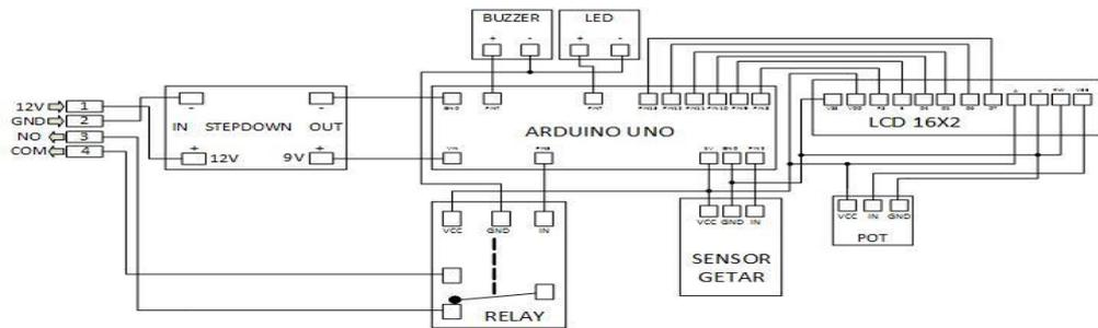
**Figure 4:** System Circuit Schema
